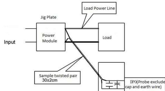
2) The test diagram is shown on the right. The converter output connects to the electronic load by the jig with cables which size should be defined according to the output current value. The twisted pair (length 30cm±2 cm) should be connected in parallel with the load, the location is as close as possible to the output pins or terminals. The test can be started after input power on.
